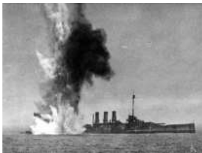
A 2,000 lb. bomb "near-miss" severely damages Ostfriesland at the stern hull plates
